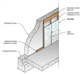
**Stud Wall Construction** - TSX-8500 may be applied to the interior face of wood or metal studs to provide a layer of continuous insulation (ci) over the entire surface. Simply secure the TSX-8500 directly to the framing members. For example, TSX-8500 is an outstanding product for use in insulating the walls or ceilings of attics and crawl spaces. Consult your local Building Code for ventilation requirements within attics and crawl spaces.
