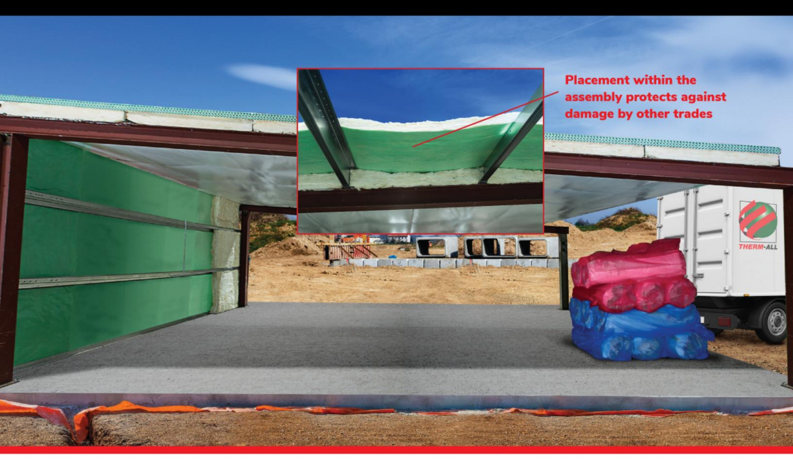
The patented system consists of a vapor retarder, at least one layer of fiberglass, and a continuous air barrier. The air barrier material is a cross-woven non-perforated building wrap with a breathable polyolefin coating, and is designed to perform as both a water-resistive barrier and as a breathable air barrier. A perm rating of 25 allows water vapor to pass through the air barrier so that moisture isn't trapped between the vapor retarder and the air barrier.
