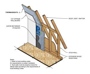
**Attics and Crawl Spaces** - Thermasheath-3 may be applied to the interior face of stud walls or roof rafters within attics and crawl spaces to provide a layer of continuous insulation (ci). Simply nail the Thermasheath-3 to the framing members and cover with an approved ignition barrier such as 3/8" gypsum wallboard or 1/4" wood structural panel, particle board or hardboard.
