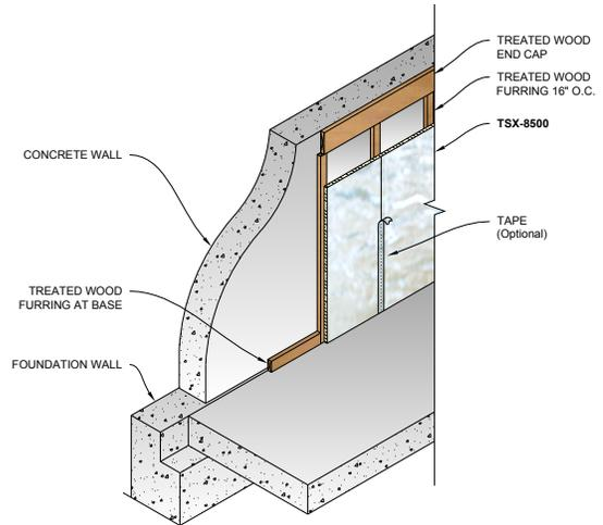
**Stud Wall Construction** - TSX-8500 may be applied to the interior face of wood or metal studs to provide a layer of continuous insulation (ci) over the entire surface. Simply secure the TSX-8500 directly to the framing members. For example, TSX-8500 is an outstanding product for use in insulating the walls or ceilings of attics and crawl spaces. Consult your local Building Code for ventilation requirements within attics and crawl spaces.
