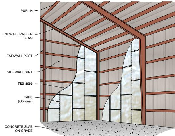
**Agricultural, Farm, Storage Buildings and Other Light Commercial Structures** - TSX-8500 is **pressure washable\*** and may be used as an exposed, finished, continuous insulation (ci) system in agricultural, farm, storage buildings and other light commercial structures where local Building Codes will permit such use.
