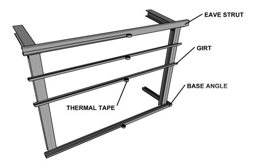
3. If a double layer wall system is required, install the outer layer of fiberglass insulation between the girts and metal wall sheets. No thermal break foam tape is required for a double layer application.
