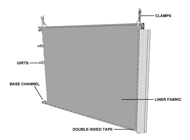
3. Move to the base angle and begin removing the tape's liner in the center of the wall section, moving towards both edges while pulling and squaring the fabric and seal to the tape. Move up both sides of the fabric, then across the top edge following these same steps. Remove c-clamps during this process while making sure the fabric is tight and smooth.
