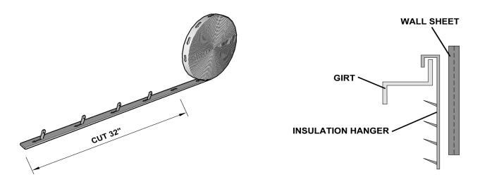
5. Two (2) hangers should be used to hold any insulation blanket up to 72" wide by placing them 18" from each side of the insulation blanket (or 36" apart). Repeat this step for each wall area to be insulated. Hangers not supplied for girt spaces 24" or less.
